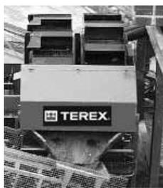
Rubber lined chute on discharge.
