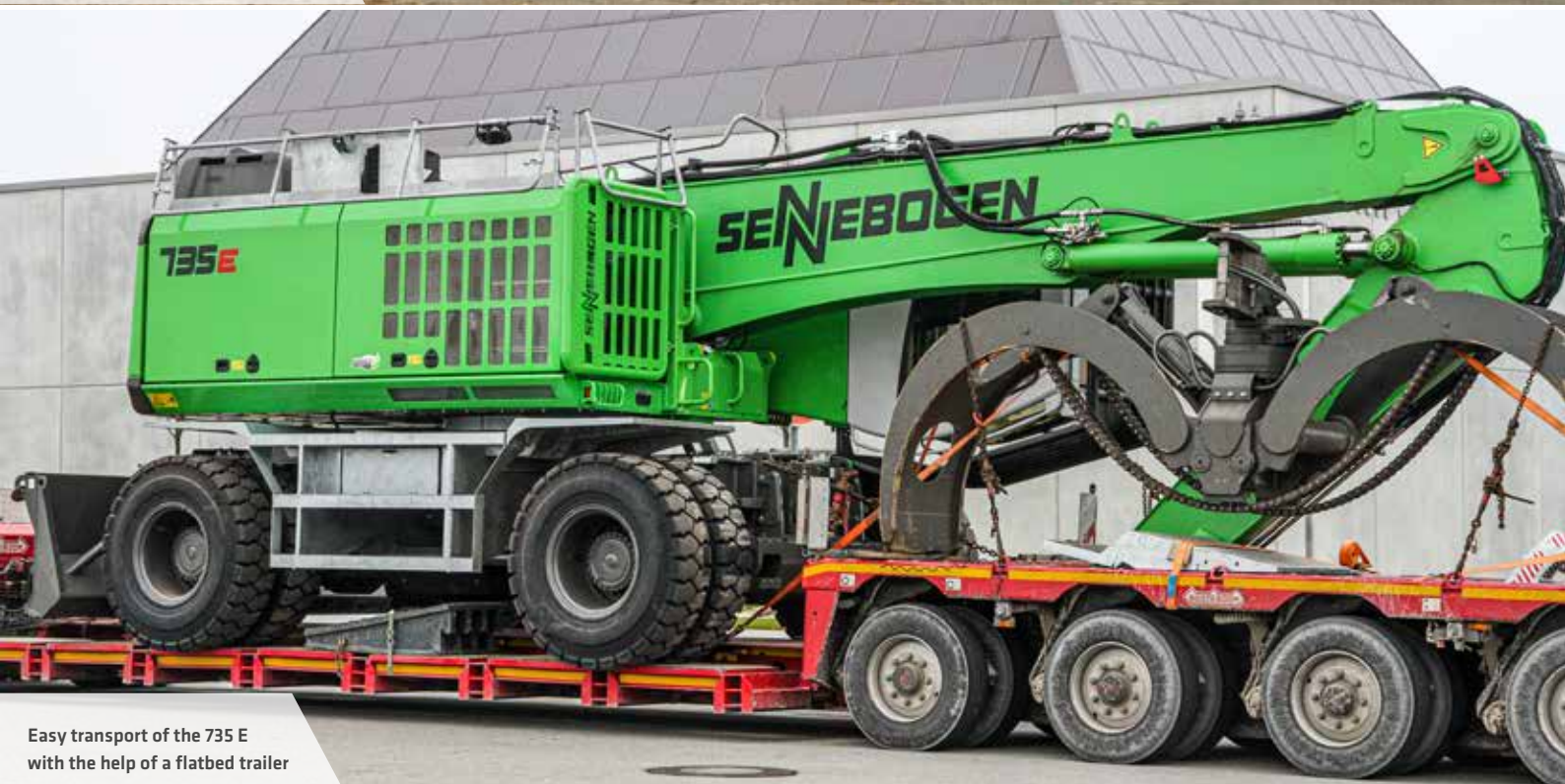
Pick & Carry operation with trailer up to 30 tonnes
