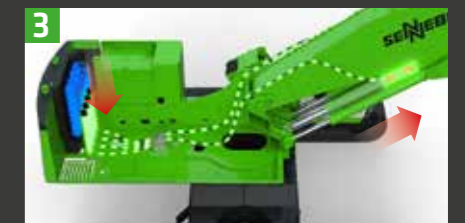
3 The nearly constant force transmission throughout the cylinder cycle supports the next boom lift
