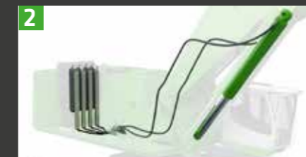
2 Energy storage module consisting of nitrogen accumulators
