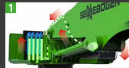
1 Boom lowers, gas compresses
