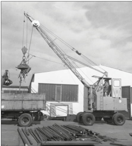
1962: rope-driven S833 with elevated operator cab
