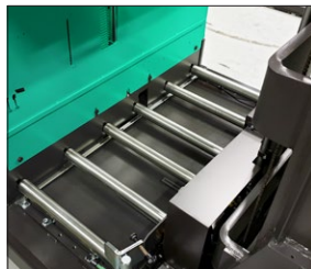
Battery on steel rollers
