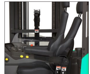
Suspension seat with tilting backrest
