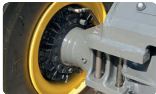
Axle oil cooling system
