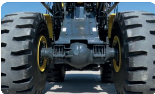
Reinforced axles and reinforced front frame
