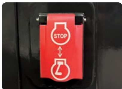
Secondary engine shutdown switch
