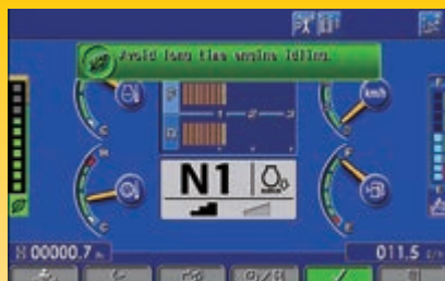
Eco-gauge, Eco guidance and fuel consumption gauge
