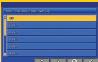
Adjustable idle shutdown automatically turns off the engine after it idles for a set period of time
