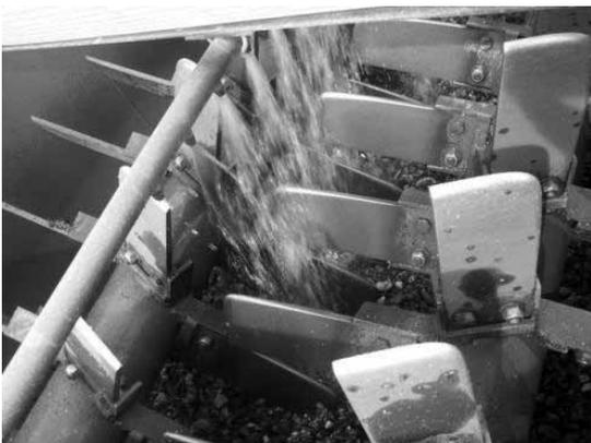
Spiral design axles with high tensile and quickly replaceable blades
