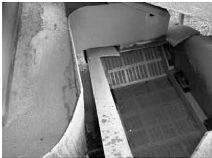
Sloped back panel and modular screen decks
