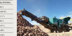
Engines are available that are certified to US EPA and EU off road diesel emission standards. Talk to your dealer about possible certification options (i.e. Tier 3/Stage 3A:, Tier 4i/Stage 3B:, Tier 4F / Stage 4).
